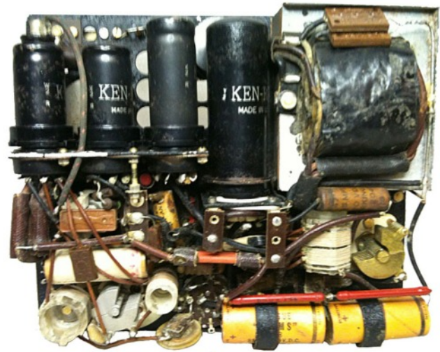
Underside view of the A 1 showing the compactness of the radio. Most of the components were imported from the USA.
