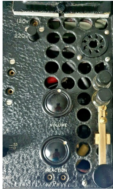
Detail photo of an A 2 showing the Morse key with two terminals of connecting an external Morse key, headphone socket, reaction control, (RF) volume control, octal power socket, AC mains selector and crystal socket.
