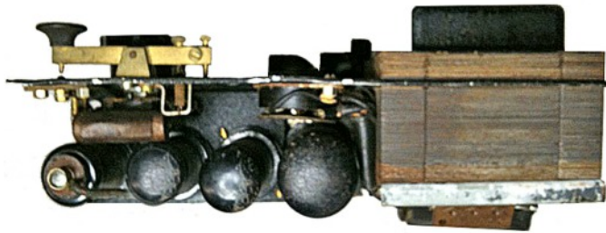
Top side view of the A 1 removed from its enclosure, showing the four steel valves, mains transformer and the mechanical construction of the Morse key.
